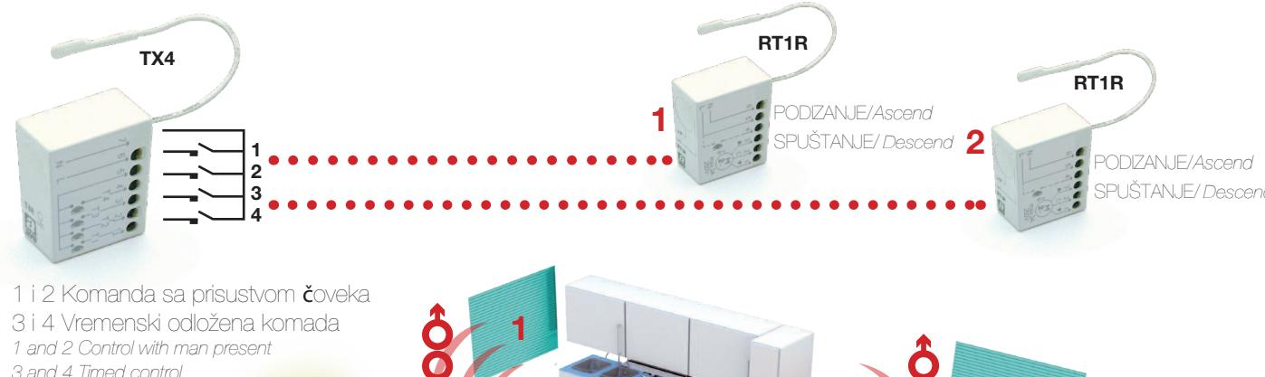
The T4R transmitter has four inputs to which normal N.O. buttons can be connected to send radio commands to the R1R receiver and to RT1R receiver to control blind motors. The signals that can be sent via the 4 inputs determine the different functioning of the receivers, as follows.
